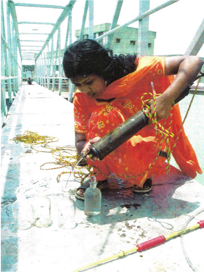
Exhibit 12.8 Collection of depth-wise samples
