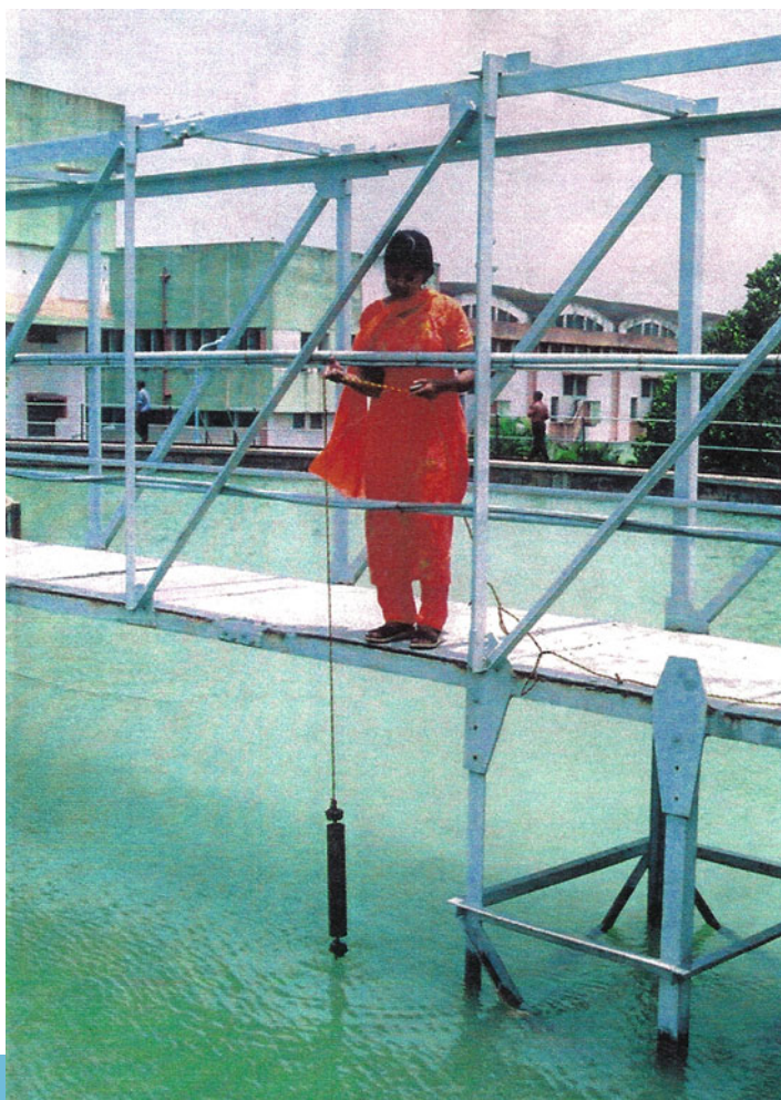
Exhibit 12.7 Depth-wise sampling using Kemmerer sampler
