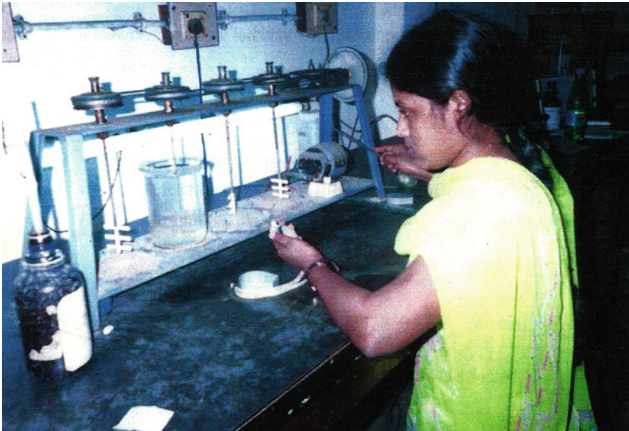
Exhibit 12.6 Setting flash mixing speed with several RPM
