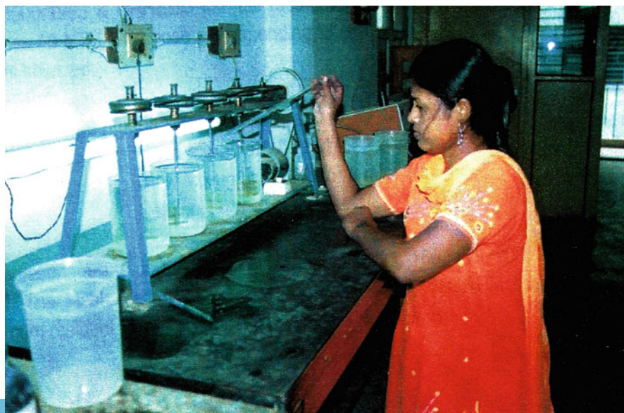
Exhibit 12.4 Jar test to determine coagulant dosage
