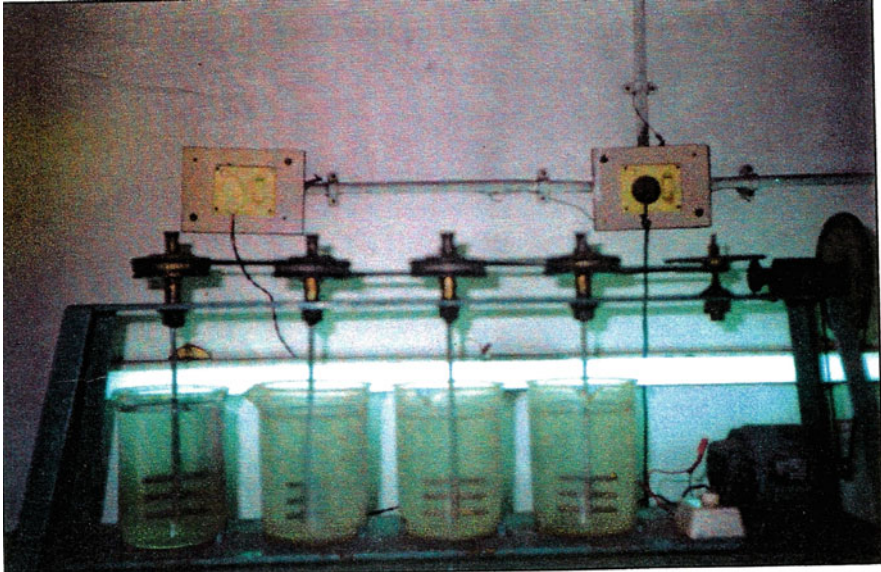
Exhibit 12.5 Jar test with flash mixing followed by slow mixing
